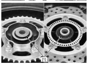
Apply grease to a new O-ring [1].
