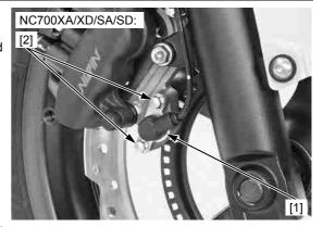
NC700X/S: Install the front brake caliper/bracket assembly [1] and tighten new brake caliper mounting bolts [2] to the specified torque.
