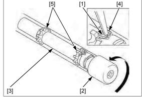
Remove the screw [1], handlebar weight [2], retainer ring [3] and rubber cushions [4] from the inner weight
