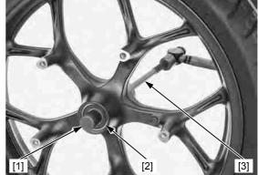
Never install the old bearing, once the bearing has been removed, the bearing must be replaced with new ones.
