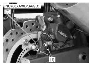
Loosen the lock nut [1], drive chain adjusting nut [2] and axle nut [3].
