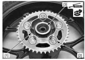
Install the pulser ring (NC700XA/XD/SA/SD) [1] onto right wheel hub.
