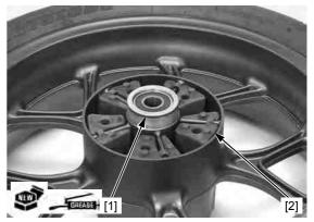
Install the driven flange assembly [1] into the left wheel hub.
