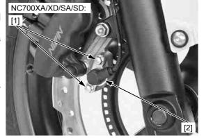
Loosen the front axle pinch bolt [1] and front axle [2].
