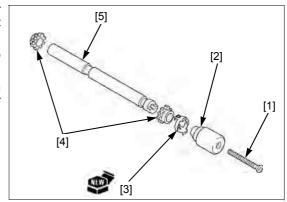
Install the inner weight assembly [1] into the handlebar. Turn the inner weight and hook the weight retainer tab [2] with the tab locking hole [3] in the handlebar.
