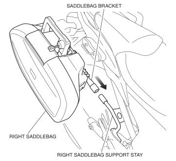
3. Insert the loop of the right saddlebag hook into the upper hole of the right saddlebag as shown.
