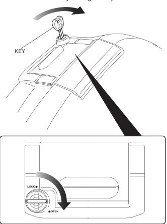
2. With the key turned clockwise, raise the plate lock and release it from the lid.
