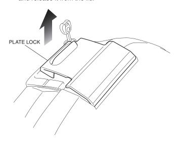
3. Open and close the lid with the plate lock released and raised.
