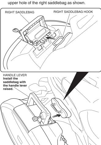
4. Lower the handle lever and lock the right saddlebag by turning the key counterclockwise as shown.
