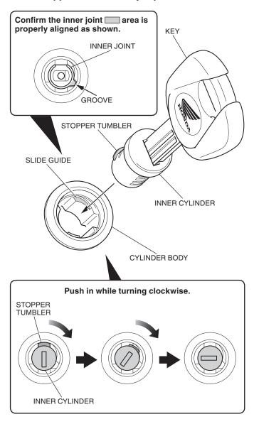
17. Draw out the key and check that the inner cylinder does not come out.
