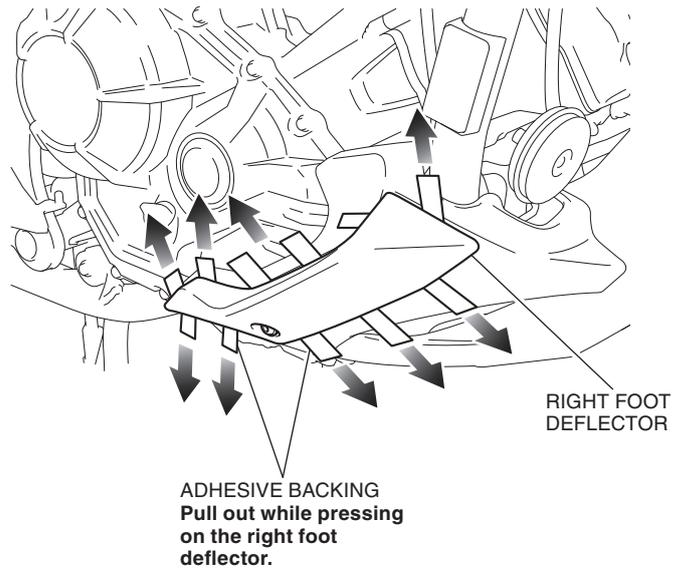
6. Apply adequate pressure to the attached right foot deflector.
