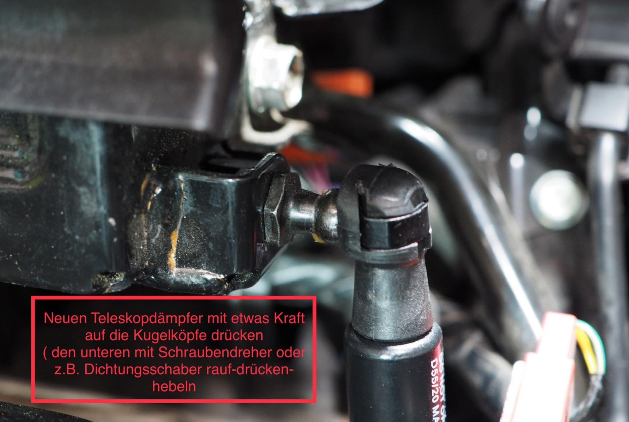
A close-up photograph of a ball joint being pressed into a new telescopic shock absorber. The ball joint is on the left, and the shock absorber is on the right. The shock absorber has a red label with the text 'DS5120 MP'. The background is dark and out of focus, showing other mechanical parts of a vehicle.
