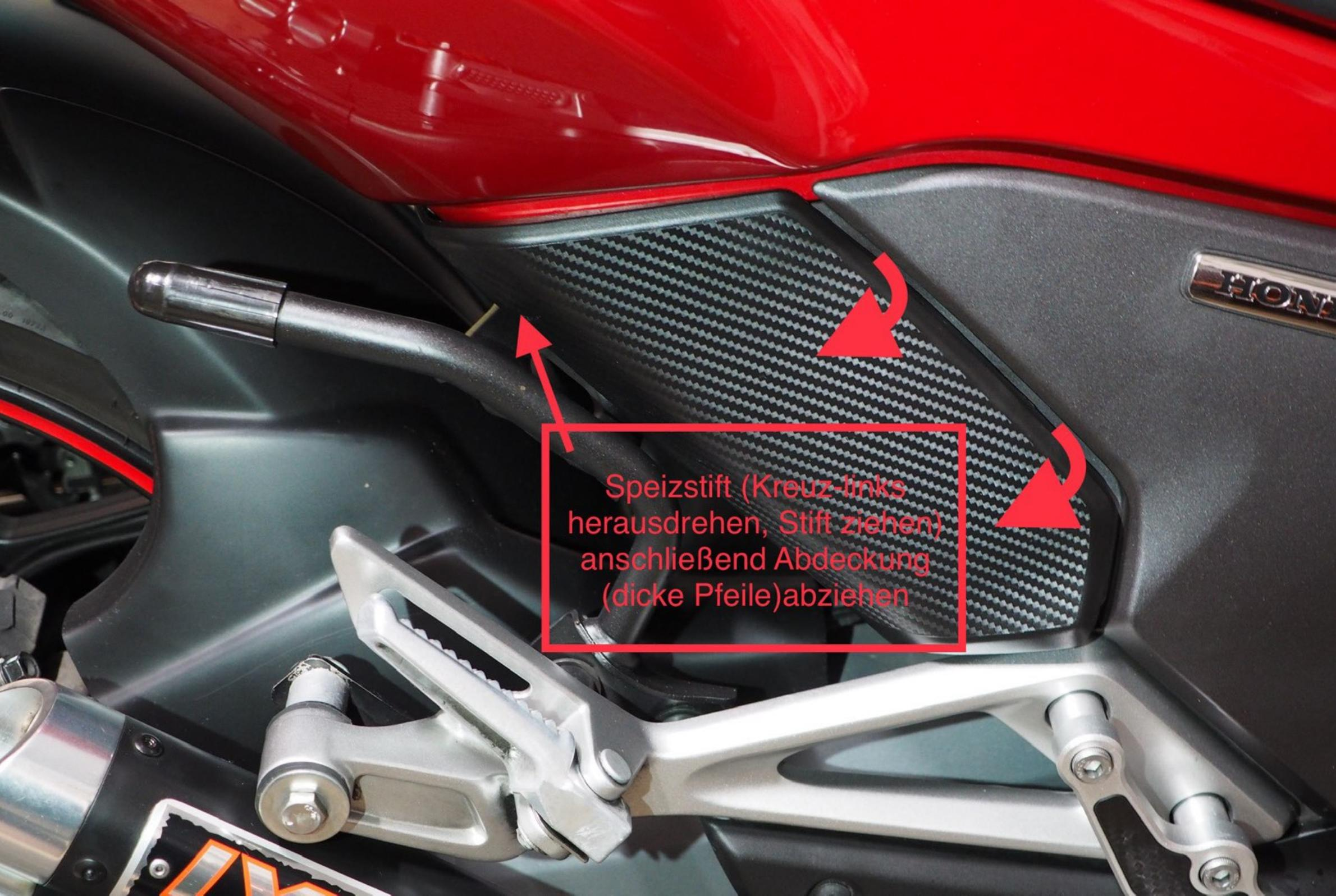
A close-up photograph of a motorcycle's footpeg area. The motorcycle is red. A black plastic cover with a carbon fiber pattern is mounted over the footpeg mechanism. A silver metal footpeg is visible. A red text box with a red border is overlaid on the image, containing German instructions. Three red arrows point to specific parts: one points to a screw on the left side of the cover, and two curved arrows point to the top and right edges of the cover, indicating where to peel it off.
