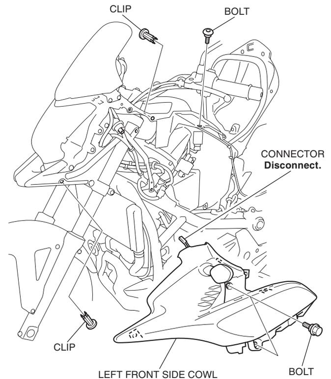
6. Release the motorcycle's 6-pin waterproof connector as shown.
