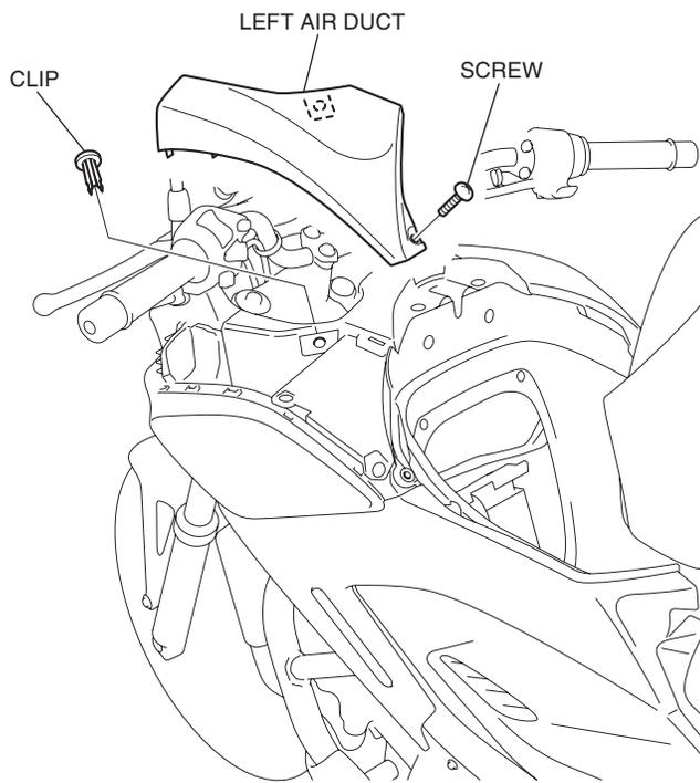
3. Remove the clip and open the front part of the left seat cowl slightly as shown.
