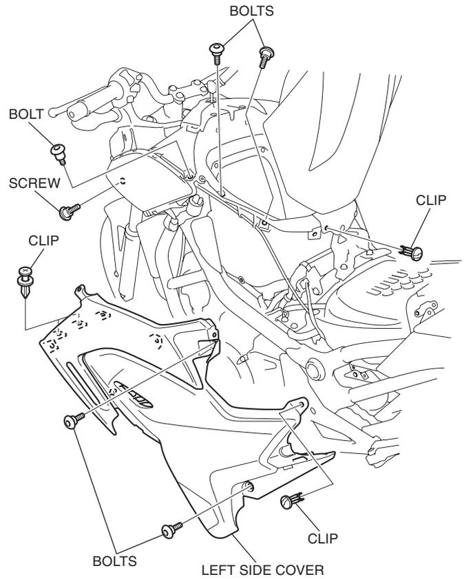
5. Refer to the Service Manual for the motorcycle, remove the left front side cover.
