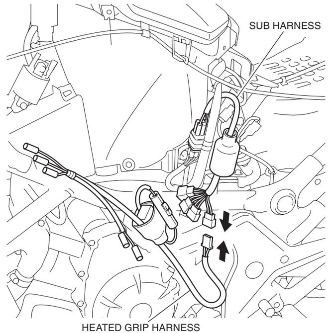
15. Cover the connectors with the harness boot as shown.
