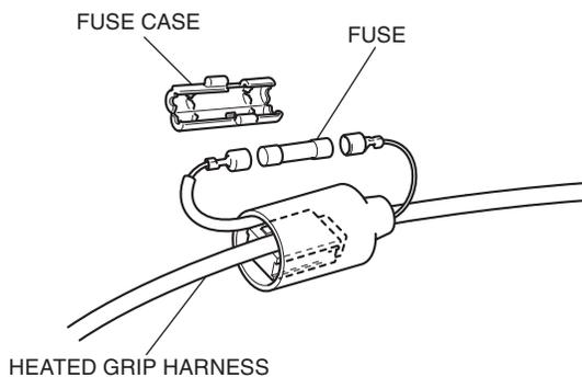
14. Connect the heated grip harness to the sub harness as shown.
