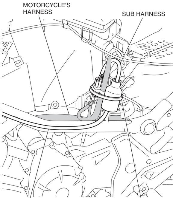
17. Route and secure the heated grip harness with the wire ties as shown.
